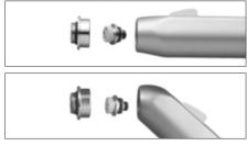
3. Remove the insert with grey o-ring from head of syringe.
