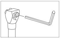
2. Unscrew and remove adapter using Allen Key. Some adapters may require a screwdriver to remove.
