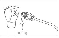
3. Verify that small o-ring is in the end of tip-adapter assembly. Screw assembly into syringe and finger tighten. Remove tip.
