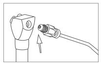
3. Verify that small o-ring is in the end of tip-adapter assembly.
