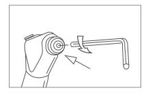
1. Remove metal tip. Using wrench, unscrew and remove tip release mechanism.
