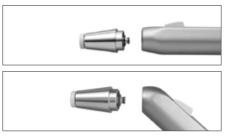
5. Screw adapter body into syringe while depressing the air and water buttons. Note: if adapter insert has separated from adapter, push insert into syringe head then screw adapter body onto syringe.
