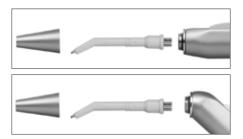
1. Unscrew original tip nut and remove tip.
